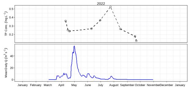
Figure 10: Mean daily discharge (m<sup>3</sup> s<sup>-1</sup>) and total phosphorus concentration (mg L<sup>-1</sup>) over the 2022 sampling season at Boyne River near Roseisle (05OF011).
