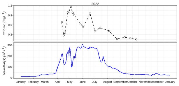
Figure 24: Mean daily discharge (m³ s⁻¹) and total phosphorus concentration (mg L⁻¹) over the 2022 sampling season at Assiniboine River near Headingly (05MJ001).
