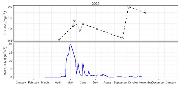
Figure 4: Mean daily discharge (m<sup>3</sup> s<sup>-1</sup>) and total phosphorus concentration (mg L<sup>-1</sup>) over the 2022 sampling season at La Salle River at Elie (05OG008).
