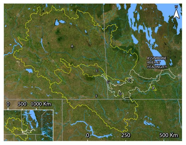
Supplemental Figure 4: Incremental drainage area in white and upstream drainage areas in yellow. Incremental loads are calculated by subtracting gross "Assiniboine River near Brandon" (A), "Cypress River near Bruxelles" (B), "Little Souris River near Brandon" (C), "Medora Creek near Napinka" (D), "Plum Creek near Souris" (E), "Souris River at Melita" (F), and "Stony Creek near Broomhill" (G), from "Assiniboine River near Headingly" values.
