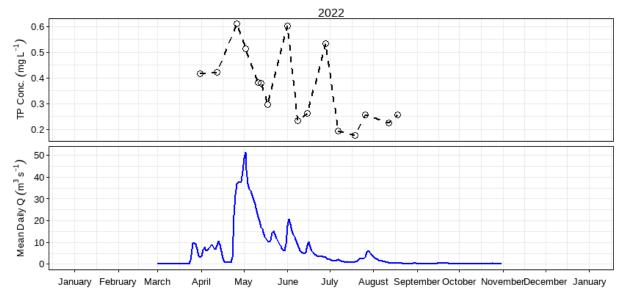
Figure 8: Mean daily discharge (m<sup>3</sup> s<sup>-1</sup>) and total phosphorus concentration (mg L<sup>-1</sup>) over the 2022 sampling season at Boyne River near Carman (05OF003).
