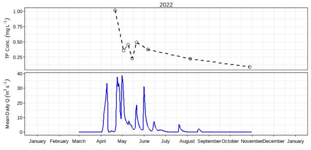
Figure 6: Mean daily discharge (m<sup>3</sup> s<sup>-1</sup>) and total phosphorus concentration (mg L<sup>-1</sup>) over the 2022 sampling season at Elm Creek Channel near Elm Creek (05OG005).
