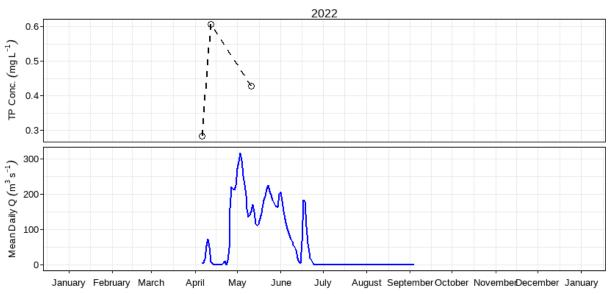
Figure 29: Mean daily discharge (m³ s⁻¹) and total phosphorus concentration (mg L⁻¹) over the 2022 sampling season at Portage Diversion near Portage La Prairie (05LL019).
