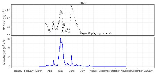
Figure 12: Mean daily discharge (m<sup>3</sup> s<sup>-1</sup>) and total phosphorus concentration (mg L<sup>-1</sup>) over the 2022 sampling season at Roseisle Creek near Roseisle (05OF009).
