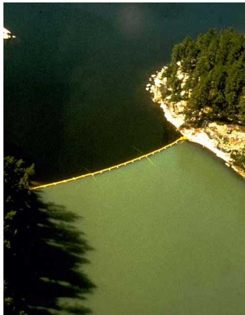
Figure 1. Lake 226 at the Experimental Lakes Area. Nitrogen and carbon are added to the top basin, while nitrogen, carbon and phosphorus are added to the lower basin. The basin with phosphorus added developed blue-green algal blooms – the other basin did not.
