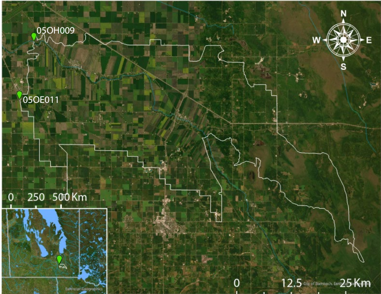
Figure 26: WSC stations 05OE011 & 05OH009 (green) and combined drainage area polygon for each respective station (white - source: 05OE011 [AAFC], 05OH009 [WSC]). LWCBMN samples directly at both WSC stations. See Supplemental Figure 4 for upstream drainage areas used to calculate incremental area.
