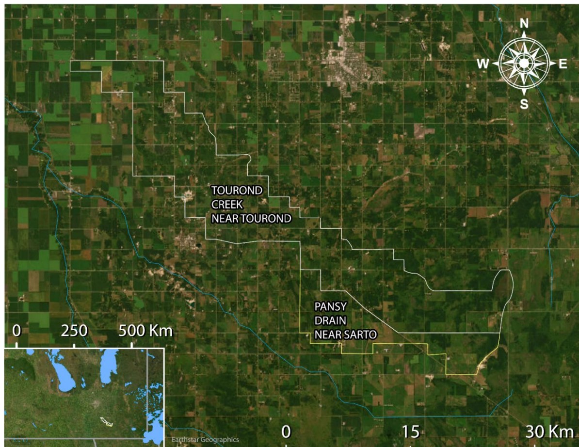
Supplemental Figure 5: Incremental drainage area in white and upstream drainage area in yellow. Incremental loads are calculated by subtracting gross “Pansy Drain near Sarto” values from gross “Tourond Creek near Tourond” values.
