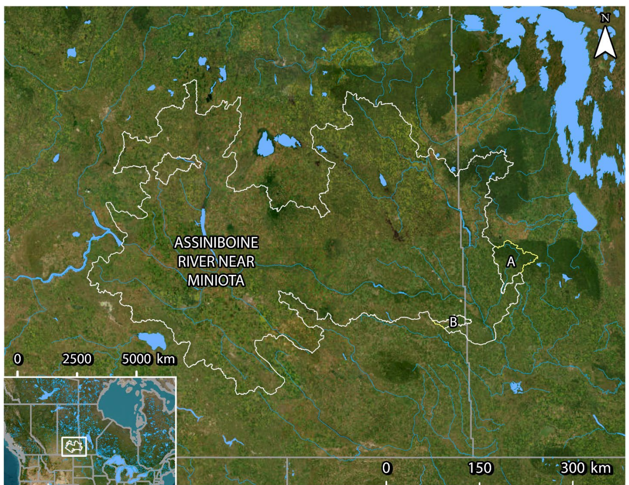
Supplemental Figure 2: Incremental drainage area in white and upstream drainage area in yellow. Incremental values are calculated by subtracting “Birdtail River near Birtle” (A – 05ME003) and “Scissor Creek near McAuley” (B – 05ME009) from gross “Assiniboine River near Miniota” (05ME006) values.
