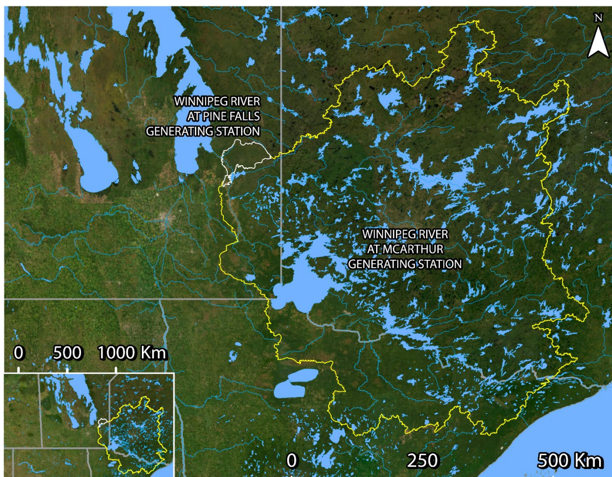
Supplemental Figure 1: Incremental drainage area in white and upstream drainage area in yellow. Incremental loads are calculated by subtracting gross “Winnipeg River at McArthur Generating Station” values from gross “Winnipeg River at Pine Falls Generating Station” values.
