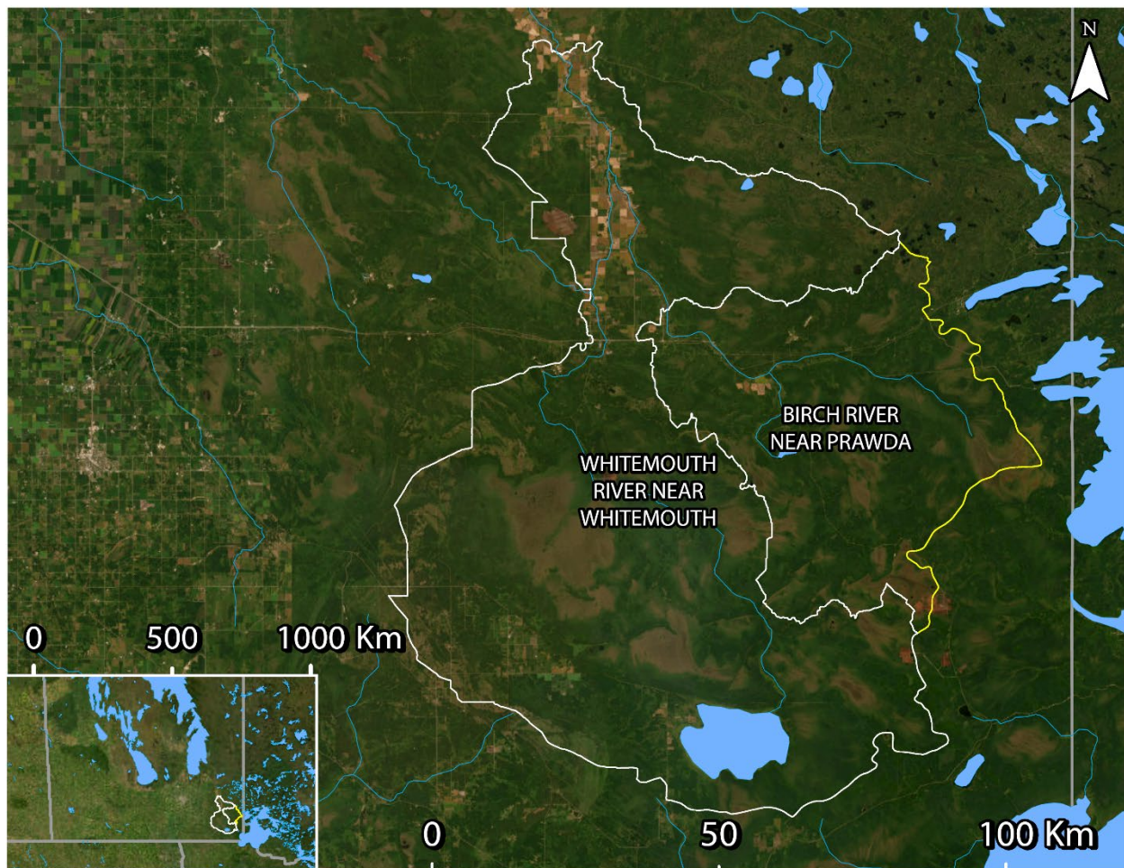
Supplemental Figure 3: Incremental drainage area in white and upstream drainage area in yellow. Incremental loads are calculated by subtracting gross “Birch River near Prawda” from “Whitemouth River near Whitemouth” values.
